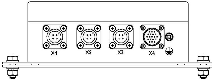
X1 - port for connection of vibration-seismic SE;
